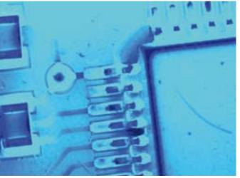
Conformal coating survey with external UV illumination besides production chains
