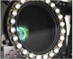
Material science for making online research measurements, the mobile floor stand is equipped with a big telecentric lens and a customised illumination for making distortion less images with a Megapixel Camera
