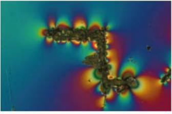
Stress measurement with polarisation and DIC techniques on glass and plastics
