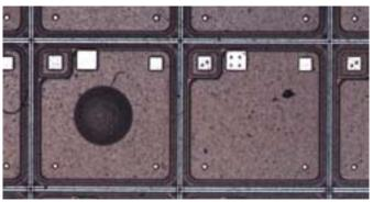
Ink dots on Wafer dies can be selected and identified with EPI coaxial Illumination and Laser injection
