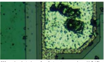
500x semiconductor image for adjustment purposes done with Epi fibre Illumination and Laser injection
