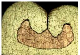
Stereoscopic measurement solution for quality control on electrical parts like crimped wires as well as the possibility to use attached prober needels.
