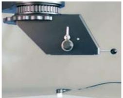
The adjustment of the working angle is easily accesible using the small lever on the side
