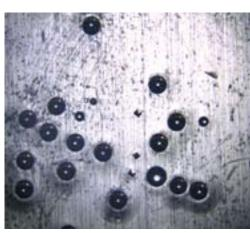
Measurement of holes, scratches and defects on large sheets in production environments.
