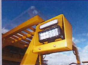
Highly visible LED lamp installed
