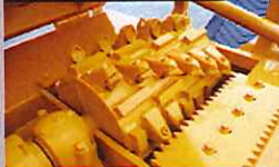
Hammer type cutter drum
