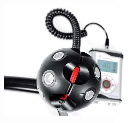
The SONOSPHERE mobile ultrasonic system provides quick and reliable detection of seal failures in windows, doors, cabins, vehicles and containers which have sealing surfaces or rubber profile seals.
