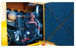
**ENGINE.** The TR620 features a Cummins QSB 3.31 Tier 4i (Stage IIIB), 120 hp (90kW) engine. The engine is mounted on a pivoting frame that swings out 30 degrees for superior access to fuel filters and hydraulic reservoir for maintenance and service.
