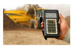
**CONTROL SYSTEM.** Operators can control the machine through either the Vermeer DP10 display mounted on the control panel, or through a hand-held transceiver remote. From either control, the operator can choose from four programmable presets or adjust on the fly based on the incoming material.
