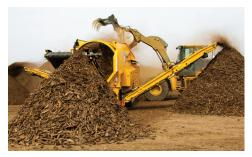
**THREE-PRODUCT CONFIGURATION.** With the flexibility to choose an optional three-conveyor configuration, the TR620 allows you to extract three unique products from the incoming material.
