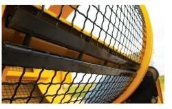
**TENSIONED SCREENS.** With the ability to tension the screen around the drum, operators can add rigidity to the screens. This design allows the use of smaller gauge wire, ultimately increasing the open area of the screen to help improve productivity.
