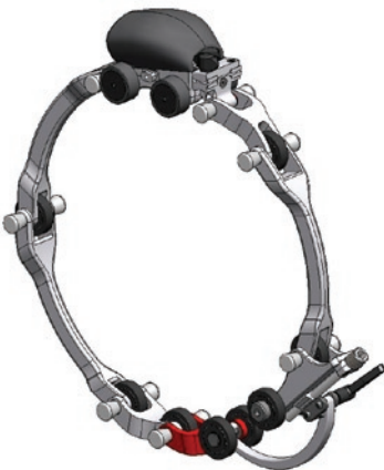
Probe-positioning system with lead screw adjustment
