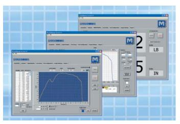
The program includes a set of tools to analyze test results, including statistical calculations, quick data export to Microsoft Excel, customizable reports, pass/fail indicators, and many others. Test setups and sequences are customizable and can be saved and recalled. The user can program test start and stop conditions, including load, time, distance, and sample break.
