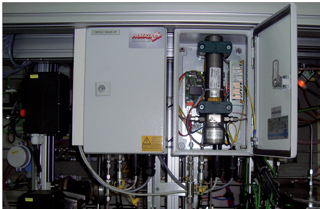
Due to its compact design, the online particle counting system PAMAS 4132 can be easily integrated into existing test rigs.
