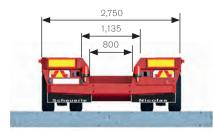
Wide and very deep prism boom recess without any narrowing (550 mm above the road surface)
