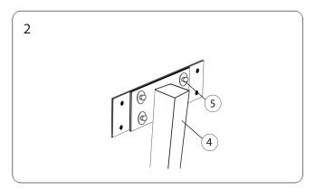
Fit the fixings through the matching holes in the post (Item 4). Securing them with washers and nuts (Item 5).
