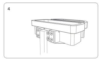
Fit the fixings through the matching holes in the post (Item 4). Securing them with washers and nuts (Item 5).
