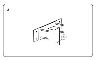
Fit the fixings through the matching holes in the post (ITEM 4).
