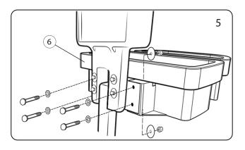
Fix the washers over the bolts and fit through the 4 outer holes in the adapter plate and then into the TSU (ITEM 6).
