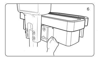
Secure in position with washers and Nuts.
