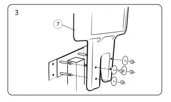
Locate the Sign Carrier's (ITEM 7) fixing holes on to the exposed bolts protruding through the rear of the Post.
