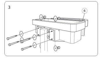
Attach the TSU (Item 6) by fitting the washers over the screws and fit through the 4 outer holes in the adapter plate and then into the TSU.
