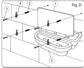
**NOTE:** Instructions are for fixing to a masonry wall. Other wall types should be assessed for the most appropriate permanent fixing method.
