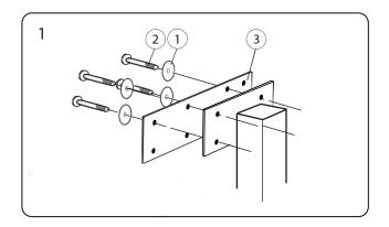
Fit the washers (ITEM 1) over the screws (ITEM 2) and fit through the 4 central holes in the adapter plate (ITEM 3).
