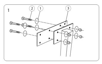
Fit the washers (Item 1) over the screws (Item 2) and fit through the 4 central holes in the adapter plate (Item 3).
