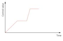
Standard programs include testing at a constant speed, as well as testing where the controlled parameter is increased at a constant rate, and then held at a certain value. The controlled parameters include stroke, test force, strain, and others.
