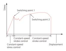
A tensile testing control program for metallic materials (JIS Z2241 and ISO 6892-2009) is included standard.
