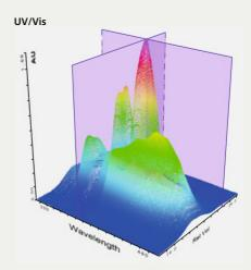
The **UV/Vis photodiode array** (PDA) covers wavelengths of 190-900 nm, opening up absorbance measurements to a wider application range.
