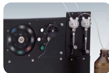
...reagent injection and fast filter switching
