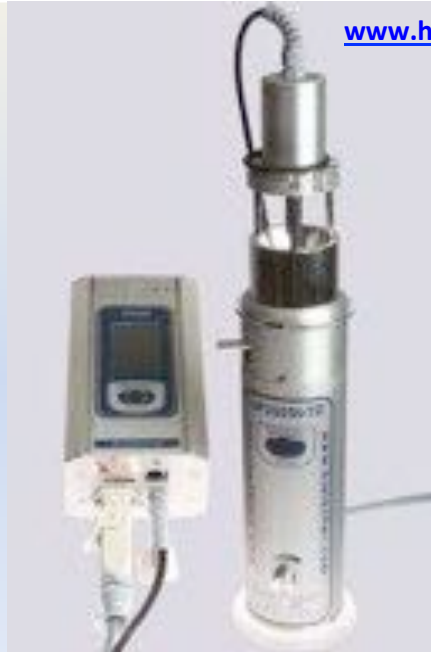
generator UP200St + transducer TD + top piece SonoStep
