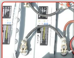
**BATTERIES :** Gel 2 x 12V/66A (C5)
