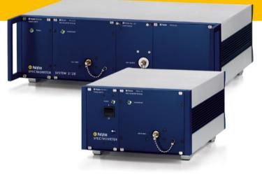
PSS spectrometers offer an optimal solution for NIR process analytics. Based on diode array technology combined with superior transmission grating design, PSS spectrometers are used for fast and reliable data acquisition. The use of fiber coupled probes enables flexible integration in various measurement scenarios.
