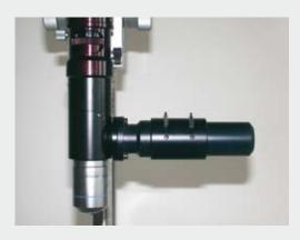
Köhler allows homogeneous illumination and increased control over the contrast and depth of field of the image.
