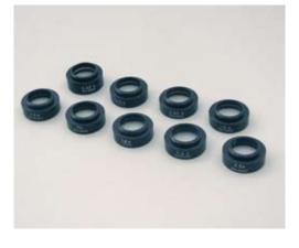
These compact objectives are optimised for their working distance and are infinity corrected. All feature standard M25x0.75 threads for compatibility with most microscopes. They fit the Multi Purpose Microscopes, Fixed Mag. and Zoom Objectives (>> page 14, 8, 10).
