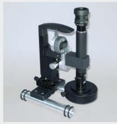
Portable Zoom Microscope with interchangeable C-Mount or eyepiece with height measurement
