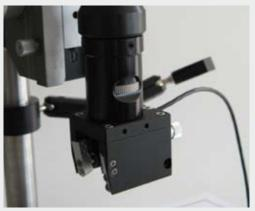
Flexible mounting of microscope with 7° viewing adapter with integrated white LED illumination.
