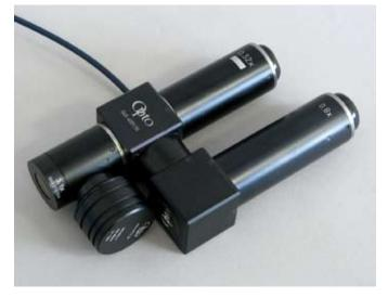
Twin field objectives are used where two different magnifications of an object have to be rapidly inspected simultaneously. This solution offers a number of benefits over zoom-based systems including: a) the elimination of magnification changing times b) elimination of inaccuracies in zoom positioning, and c) cost reduction. We can build custom solutions tailored exactly to your specific need and budget.
