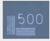
Illumination with coaxial LED Blurred picture, low contrast
