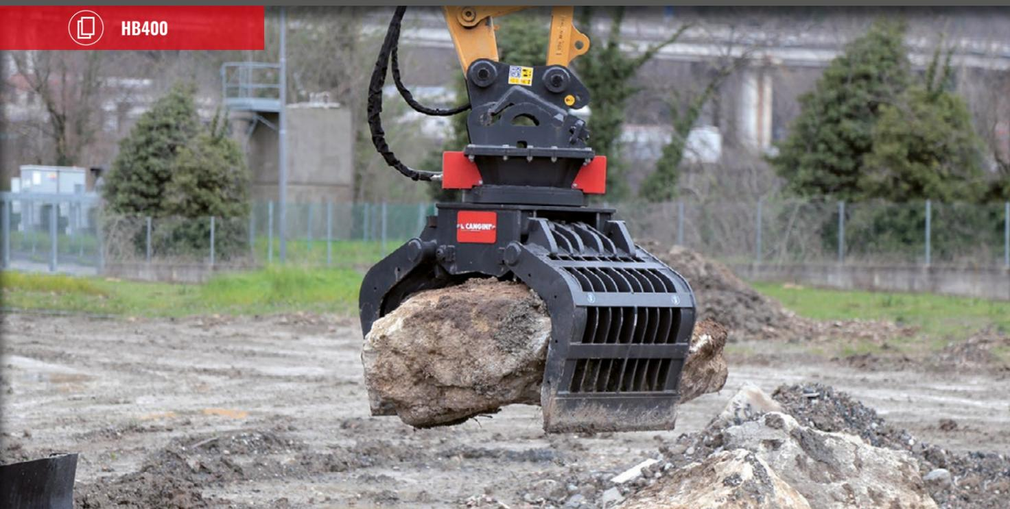
ROTATION HYDRAULIQUE POUR TOUS LES MODÈLES. CONÇUS POUR MANIPULER MATÉRIELS DIFFÉRENTS. LES PINCES SONT EN HB400 AVEC LAMES RÉVERSIBLES BOULONNÉES. LEUR STRUCTURE ROBUSTE PERMET D'EFFECTUER DES PETITS TRAVAUX DE DÉMOLITION.
