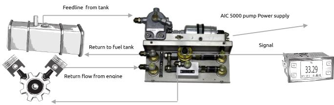
Feedline to fuel pump of the engine
