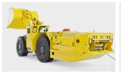
The patented cable reel control system automatically regulates tension to minimize wear on the cable and extend its longevity.
