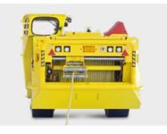
The horizontal cable reel enables a lower tension on the cable which will further improve the cables lifetime.
