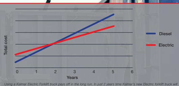
Using a Kalmar Electric Forklift truck pays off in the long run. In just 2 years time Kalmar's new Electric forklift truck will break even compared to the equivalent Diesel truck.
