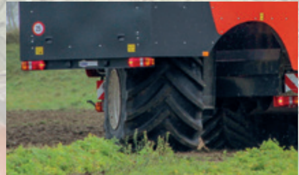
Optional super-wide rear wheel (1250/50 R32) with a tyre pressure of 0,9 bar.
