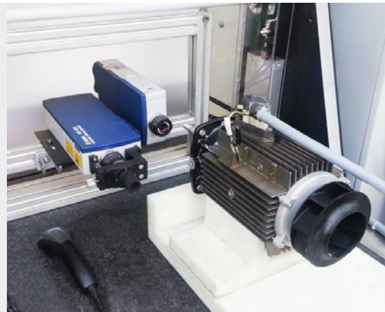
Reliable non-contact end-of-line testing on single components or complete assemblies (here on a WILO heating pump using two industrial vibrometers).
