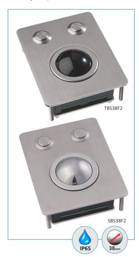
This range of compact trackball units is highly ruggedized and designed for harsh industrial applications, kiosk consoles, navigation controls, etc... They feature a robust, vandalproof construction and all metal look: the carrier plate made of brushed stainless steel, a stainless steel ring protecting the trackball sealing and anti-vandal stainless steel IP65 sealed switches.
