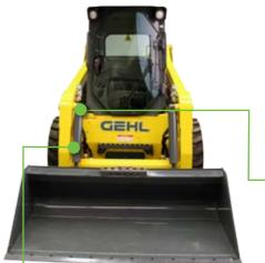
OVER-THE-TIRE design provides wider access and improved visibility. On the R220 and R260
