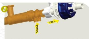
After sterile media transfer is complete, simply press the thumb latch and pull the valve back into the steam position. The "CPC **Click"** confirms the transition is complete.
