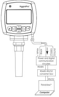
Digital communications wiring connection and networking capability
