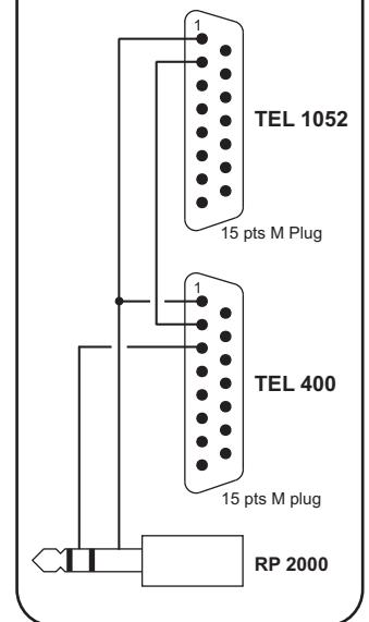
Wiring with a mixing desk without Hybrid specialised input.
