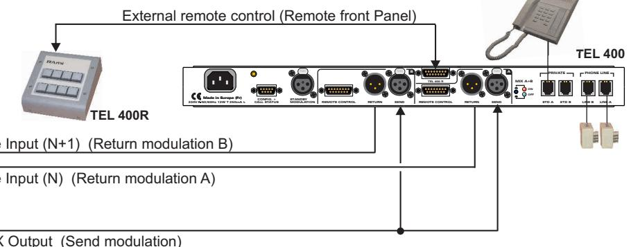
Note : if the mixing console features to AUX output, it is possible to separate « Send » to A and B hybrid.
