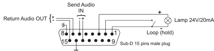
**G)** 15 pins female Sub-D 15 for use with remote control TEL 400R (or with RP2000)
