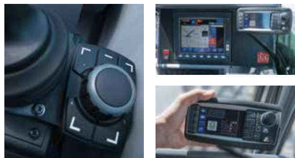
Rotary-push button, main and removable additional display.
