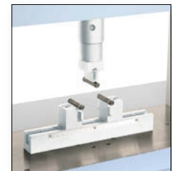
3-point bending test of plastic specimen
