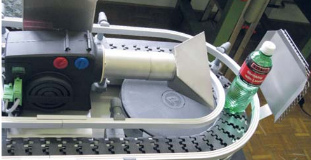
HOTWIND SYSTEM with wide slot nozzle integrated in a blow-off application.
