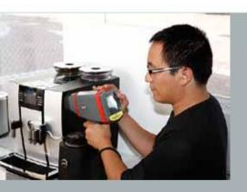
THIS HANDHELD ENERGY DISPERSIVE X-RAY FLUORESCENCE (EDXRF) SPECTROMETER
