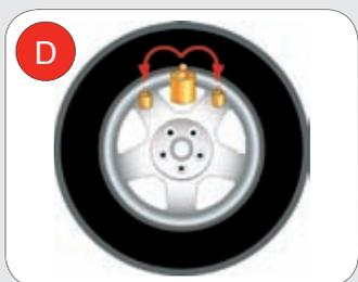
**(EN) HIDDEN WEIGHT AND SHIFT PLANE PROGRAMS (ALU P):** "Hidden weight" subdivides the external adhesive weight in 2 parts to be positioned behind the spokes of the rim. The patented "Shift Plane" program calculates the balancing position to allow using commercial adhesive weights.
