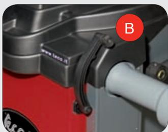
**(EN) INTERNAL DIGITAL GAUGE:** Automatic acquisition of wheel distance and rim diameter spin parameters (max diameter measurable with internal digital gauge 28", manually settable 35"). External gauge TE66 available on demand to automatically store also the wheel width parameter.
