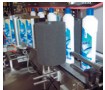
Rulli adattatori AS01 Adapting rollers AS01. Rouleaux adaptateurs AS01
