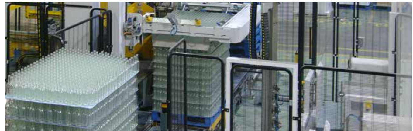
Pneumatic grippers which hold back the pad as the layer advances
