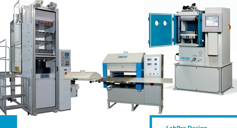
The Fontijne laboratory Platen Presses are being used in the polymer processing, rubber, and composites industry. The presses are utilized as sample preparation equipment for: Quality control, Research and Materials development.
