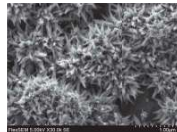
FlexSEM 5.00kV x30.0k SE Accelerating voltage: 5.0 kV, Magnification: 30,000x Specimen: hydrogen storage alloy
