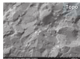
Accelerating voltage: 15.0 kV, Magnification: 500x, Specimen: varistor
