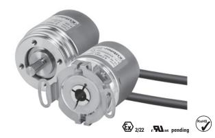
The Sendix F36 multiturn is an optical multiturn encoder in miniature format, without gears and with 100% insensitivity to magnetic fields. With a size of just 36 x 42 mm it offers a through hollow shaft of up to 8 mm or a blind hollow shaft of up to 10 mm.
