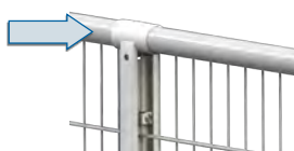
Rupture main courante
