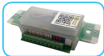
Three Phase Power monitors embedded into OEM devices or PDUs.
