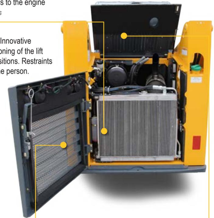
● **SWING-OUT REAR DOOR** Rear door easily opens on hinges, allowing full access to filters and fluid reservoirs for servicing and maintenance.
