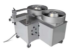
The Artos CD-17 offers coiling of large gauge wires processed on the Artos CS-327. This unit features a dual bowl system, allowing increased productivity by allowing the removal of wire from one bowl while the second bowl is being loaded. Three bowl sizes are available with quick change feature. When not in use, the CD-17 can be rolled away from the CS-327 to allow collection of shorter cables.
