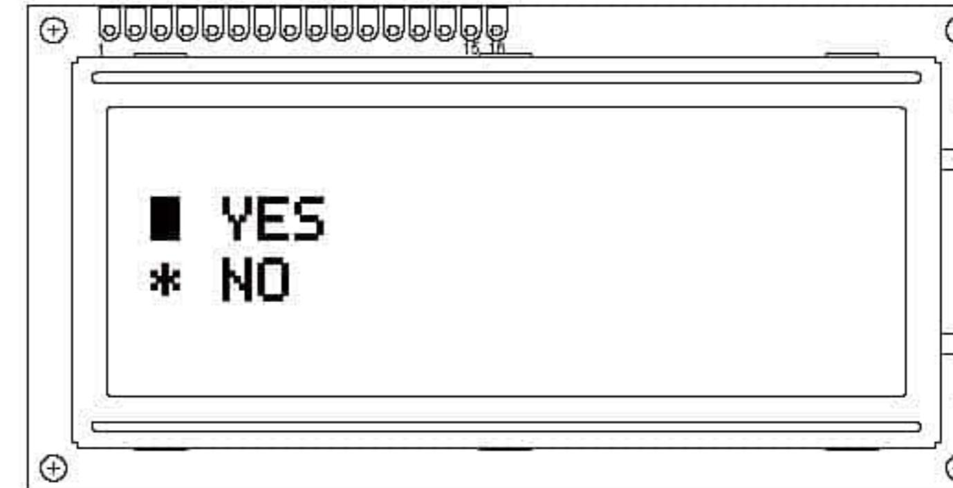
Select "YES" and press "OK" to enter the parameter setting interface. The setting time is about 1~2 minutes.
