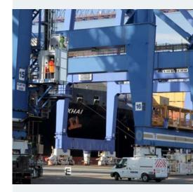
STROS rack and pinion industrial elevators are primarily used as a means of vertical access for personnel and material in various industrial facilities. They are designed to reliably perform with long life cycles in harsh environments. They are built to comply with the European Machinery Directive, or they can meet the ASME A17.1/B44 code enforced mainly in the US and Canada.
