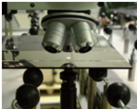
High resolution multi contrast microscope with large manual rolling table for overview and detailed inspection of large glass substrates
