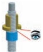
HSE type 2, compression et traction
