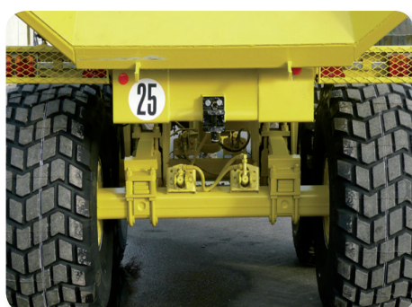
Suspension bogie Crochet arrière de traction démontable Bogie suspension Removable rear towing hook
