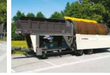
Easy access to the motor, the hydraulic system and the drum allows for ease of maintenance, cleaning and drum change.
