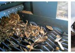
A core part of our 3-fraction-systems is the disc screen. The metal discs are not only considerably more resistant to abrasion, they can also be exchanged individually to reduce costs.
