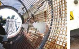
No auger in the drum, no forced conveying - in order to guarantee an optimum output quality with varied materials, the drum tilt, as well as all of the drivetrains are individually adjustable.
