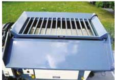
The TTS 520 can additionally be equipped with a stone grate or a vibro grate to remove large debris.
