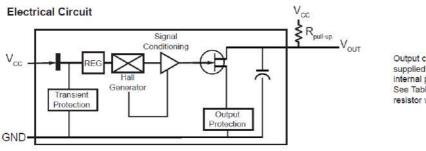
Output channels require customer supplied pull-up resistors unless internal pull-up option is selected. See Table 1.1 for recommended resistor values.
