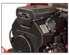
Two Kohler EFI 26.5 hp gasoline engines provide maximum power output to the rotors through electronic fuel injection.
