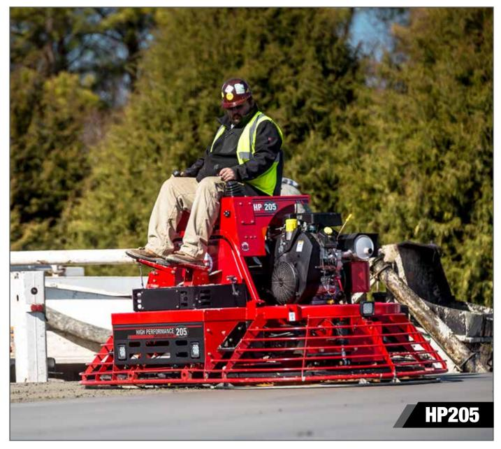
The High Performance series of riding trowels, feature twin Kohler EFI gasoline engines. These machines are workhorses built for concrete professionals to deliver maximum horse power with electronic fuel injection. Utilizing torque converter clutches, they provide excellent low speed torque for low speed float panning and superior high rotor speed for finishing concrete.
