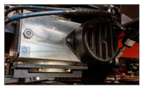
To ensure maximum energy transfer between the engine and the rotors, we equipped the HP205 with our largest gearbox (XHD).
