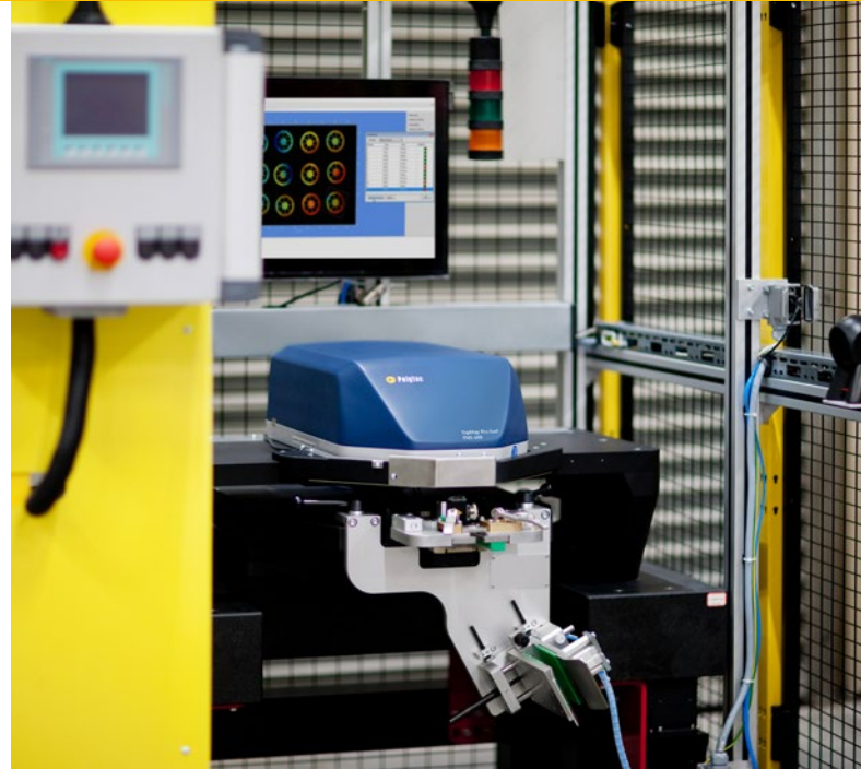
Customized solutions for in-line measurement (with integrated bar code scanner and automated sample detection)
